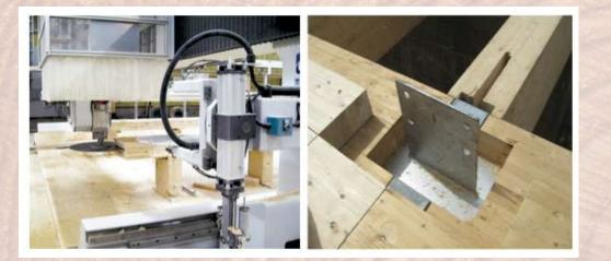
CNC machined panels and joints
